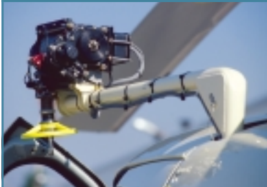
Air Equipment Electrical Hoist
