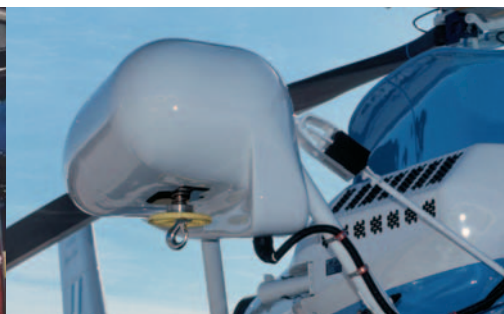
Electrical rescue hoist
