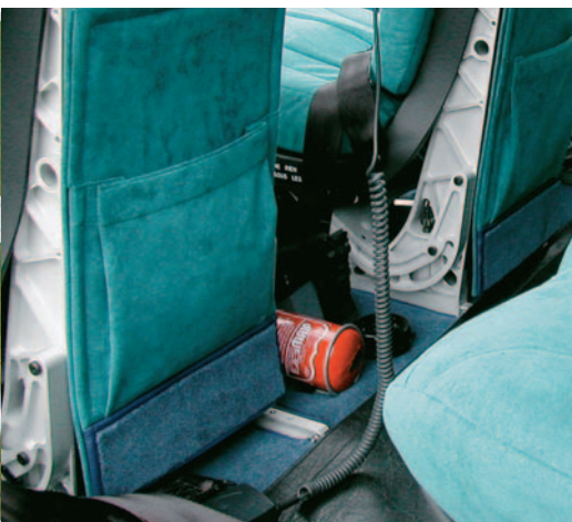
Cabin fire extinguisher
