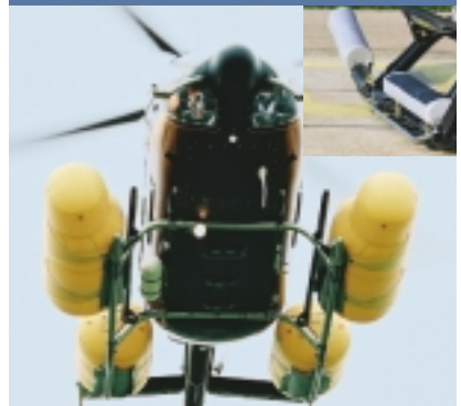
Emergency floatation system unfolded 🔴 System folded
