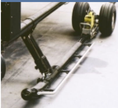
Skid protector for rescue winch cable
