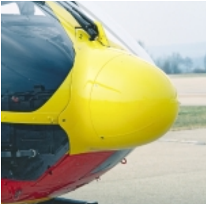
Radome integration for multimode search, rescue and weather radar
