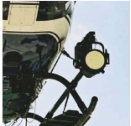
NVG compatible SPECTROLAB SX16 Search light
