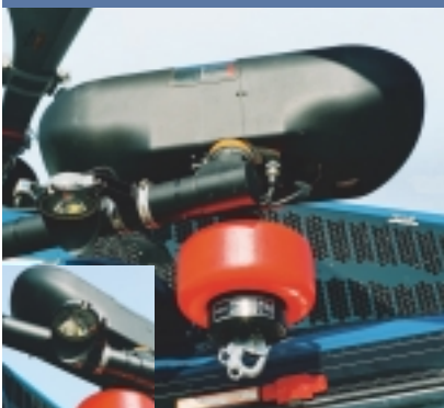
External hoist system (LH or RH) cable length = 90 m (295 ft) capacity = 270 kg (595 lb) 🔦 Rescue hoist lighting
