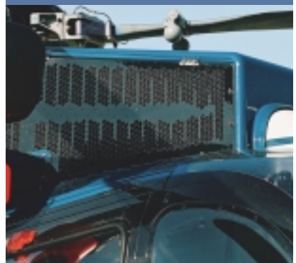
Sand filter system
